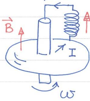
setup a circuit as shown here. The rotating disk in  $\vec{B}$  generates the current  $I$ . The current  $I$  produces the  $\vec{B}'$  field which causes feedback to the current.
