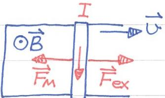
To keep the rod moving at const  $\vec{v}$ , it is necessary to apply an external force,
