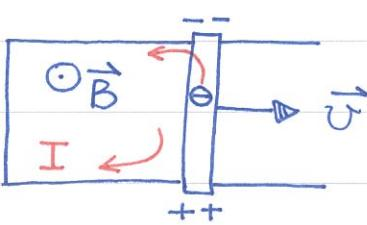
force acts on the charges in the stationary U-shape circuit but the charges near the ends of the moving rod adjust themselves to create an  $\vec{E}$  field as discussed before.
