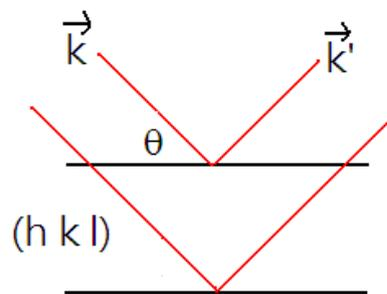
Where  $\vec{k}$  is the wave number of the incident beam and  $\vec{k}'$  is the wave number of the outgoing beam.
