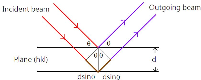
When the total path difference  $2d\sin\theta$  equals to  $n\lambda$ , diffraction occurs.
