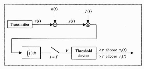
Determine the optimal threshold that minimizes the probability of error for an AWGN channel (assuming n(t) is a zero-mean white Gaussian noise with two-sided power spectral density  $N_0$  /2 and the two signals are equally probable).
