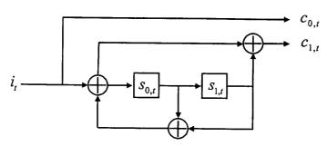
where  $i_t$ ,  $(c_{0,t}, c_{1,t})$ , and  $(s_{0,t}, s_{1,t})$  stand for the input information bit, output coded bits, and state vector at time t, respectively.
