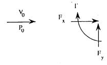
Given a vortex of strength  $\Gamma$  located at the origin in a uniform flow of velocity  $V_0$ . Show steps how to compute  $F_x$  and  $F_y$  that are necessary to maintain the vortex in equilibrium by means of the momentum theorem applied to a control volume enclosing this vortex. 20%
