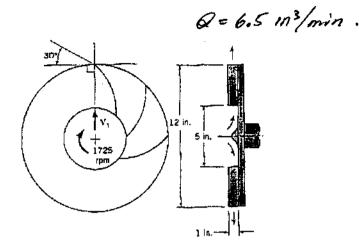
A fan has a bladed rotor of 12-in. outside diameter and 5-in. inside diameter and runs at 1725 rpm. The width of each rotor blade is 1 in. from blade inlet to outlet. The volume flowrate is steady at 6.5 m³/min, and the absolute velocity of air at blade inlet,  $V_1$ , is purely radial. The blade discharge angle is 30° measured with respect to the tangential direction at the outside diameter of the rotor. Also, in your calculations, use  $\rho_{\rm air} = 1.23 \ {\rm kg/m^3}$ .
