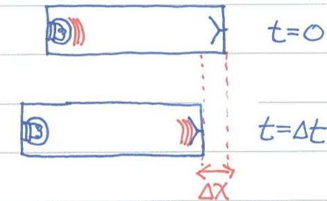
A light flash is generated at  $t=0$  and then absorbed at later time  $\Delta t$ . Because the light flash carries both energy  $E$  and momentum  $P$  (related by  $E=PC$  from Maxwell equations),
